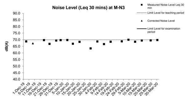
Remark: Corrected Noise Level was applied on 9 December 2019; Corrected Noise Level = Measured Noise Level - Baseline Noise Level (i.e. 67.7 dB(A))
